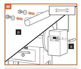
**NOTE:** Fasteners for side handle are preinstalled on handle.
