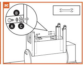
**NOTE:** Legs have a clip feature that matches up with corresponding slots on the grill body. Do not fully tighten leg bolts at this time.
