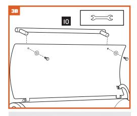
**NOTE:** Fasteners for lid handle are preinstalled on handle.
