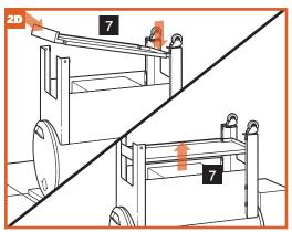
**NOTE:** After the bottom shelf is installed, fully tighten all leg bolts (Step 2C).
